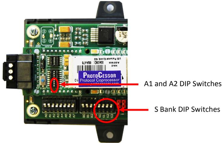
Figure 8: Location for ProtoCessor small A Bank of DIP switches
