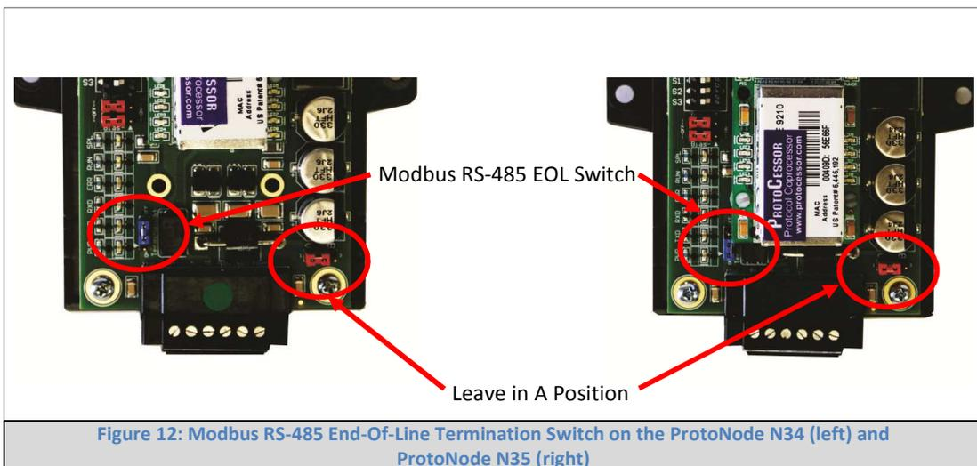
Figure 12: Modbus RS-485 End-Of-Line Termination Switch on the ProtoNode N34 (left) and ProtoNode N35 (right)
