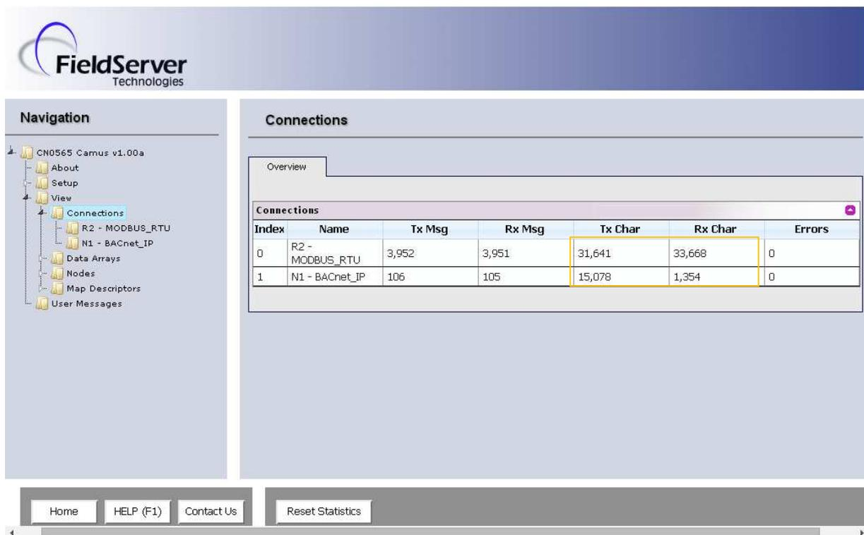
In instances, where there is more than one boiler all connected to a single Protonode it is difficult to decipher which boiler is communicating with the front end and vice versa. The web browser provides a Node Overview feature that identifies the communication that is occurring to/from each boiler.
