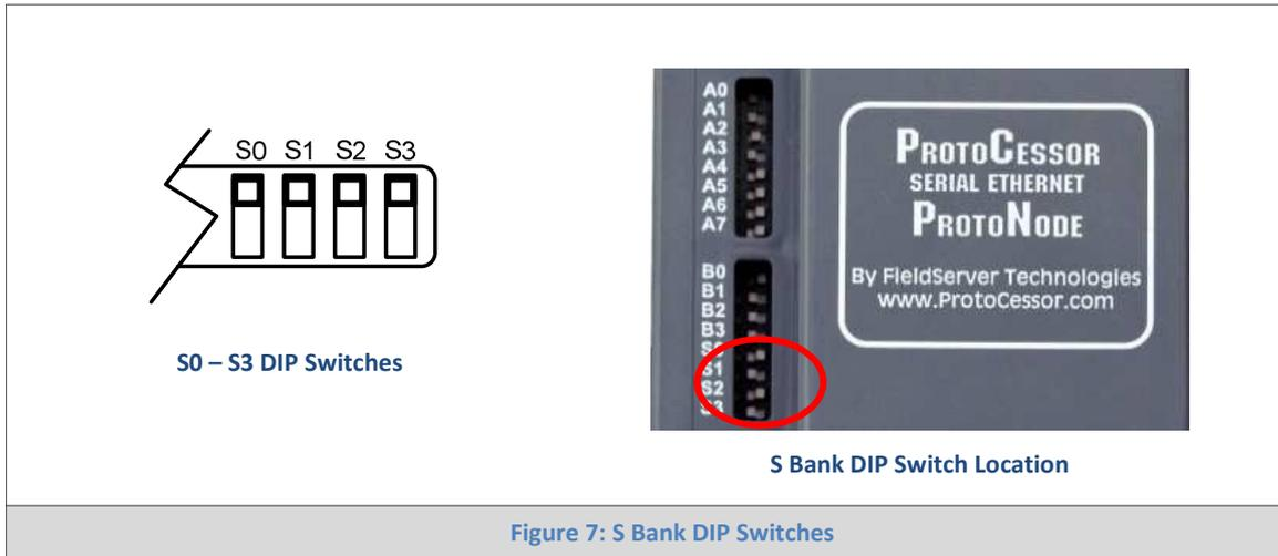
Figure 7: S Bank DIP Switches
