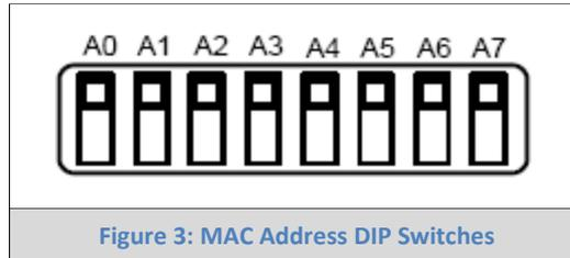
Figure 3: MAC Address DIP Switches
