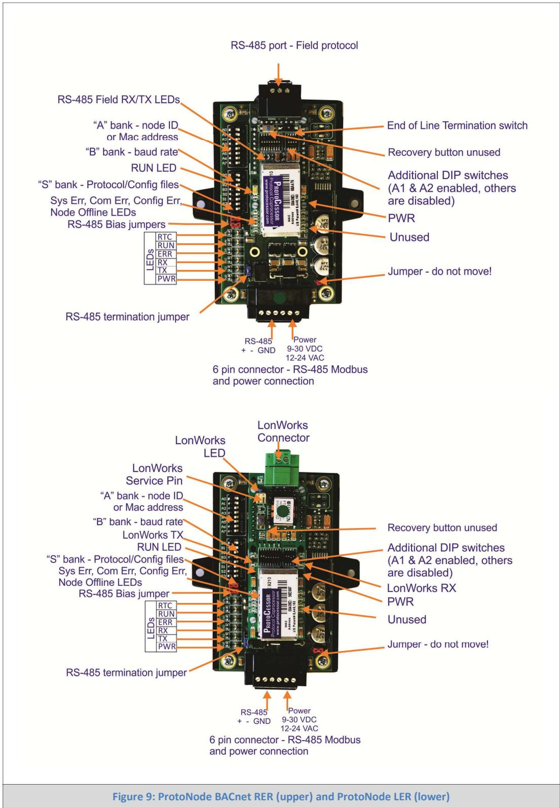
Figure 9: ProtoNode BACnet RER (upper) and ProtoNode LER (lower)
