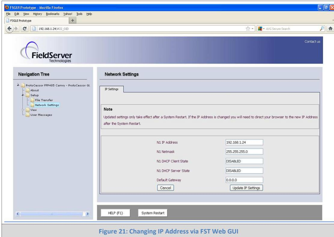
Figure 21: Changing IP Address via FST Web GUI
