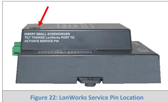
Figure 22: LonWorks Service Pin Location
